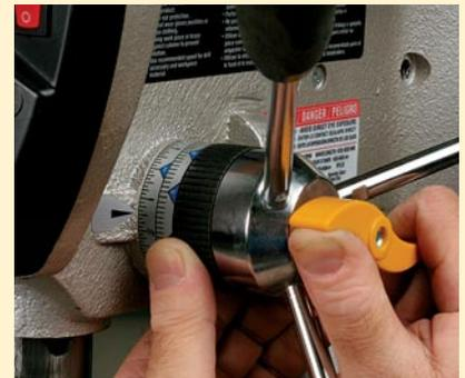
**Solid depth setting.** Seven models use stop rods for depth setting. Four of them, including the General (left) and Jet, are solidly made, with easy-to-turn, knurled depth-stop nuts. The Ryobi (above) and Craftsman have easy-to-use depth sets on their pull-arm axles.
