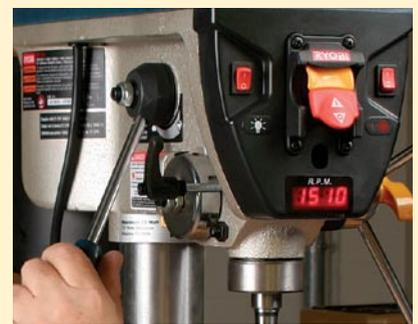
**Love that lever.** All three “best” models have a lever (left) that lets you move the motor back and forth for easy manual belt changing. The variable-speed Ryobi (above) has a digital speed display.
