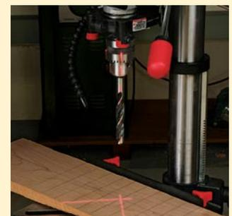
**Extras.** The Craftsman (above) is one of two models equipped with laser crosshairs. The Shop Fox W1668 (left) comes with a quill that can oscillate for spindle sanding.
